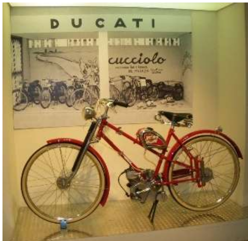
The Cucciolo , the 50cc clip-on motor that started Ducati as we know it today (bicycle extra).
